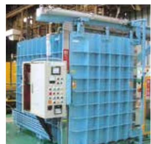
High-pressure electromagnetic switch tank
